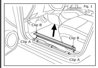
2. Place fingers at clip (A) which is located at inner rear and front end, and pull out with a slight rotating motion until clip A is popped loose, then pull up to remove door sill trim panel.
