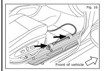
16. Place Illuminated Kick Plate into position on the driver side door sill. Feed the end of the wiring up through the existing harness clips towards the footwell.
