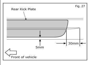
27. Place rear kick plate into position on the door sill. The rear edge should be **30mm** from the end point of the formed edge in the sheet metal of the door sill as shown. Outer edge of kick plate should be **5mm** from the outermost edge of the door sill.
