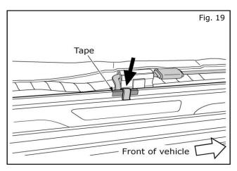
19. Cover the sheet metal edge under the wiring with a piece of foam tape. Remove all slack from the wiring at the plate end. Carefully bend the flat wire to fit tightly over the sheet metal edge.
