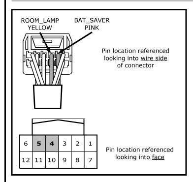
1 ) Accessory Service Connector pin-out is shown.
