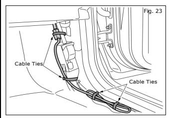
23. Plug the Accessory Connector Harness into the vehicle connector plug on the driver side.
