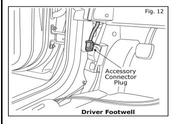
12. Locate the driver side Accessory Connector plug. It will be located below the dash along the outer wall of the footwell.
