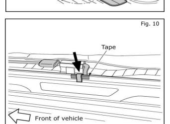
10. Cover the sheet metal edge under the wiring with a piece of foam tape. Remove all slack from the wiring at the plate end. Carefully bend the flat wire to fit tightly over the sheet metal edge.
