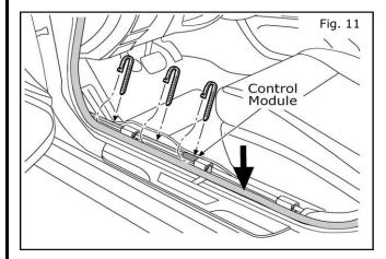
11. Press the door seal welt back down into position. Route the wires along the existing harness. Secure with cable ties as shown.
