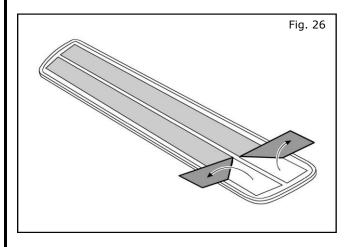
26. Carefully flip the driver rear Kick Plate over. Partially peel away enough of each adhesive liner to fold down a "flag" that will extend beyond the outer edge of the kick plate.
