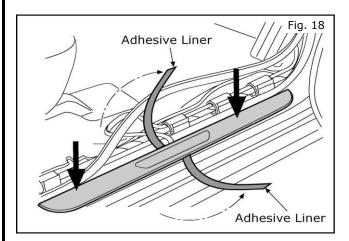
18. Carefully hold Kick Plate in position and remove the liners from the adhesive strips.
