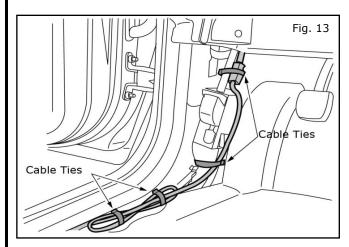
13. Plug the Accessory Connector Harness into the vehicle connector plug on the driver side.
