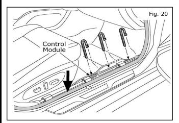
20. Press the door seal welt back down into position. Route the wires along the existing harness. Secure with cable ties as shown.
