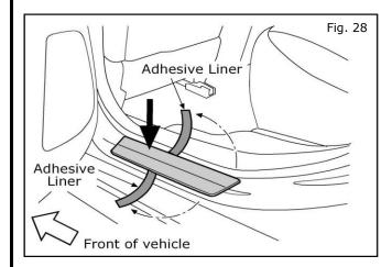
28. Carefully hold rear kick plate in position and remove the liners from the adhesive strips.
