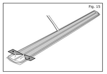
15. Carefully flip the passenger side Kick Plate over. Partially peel away enough of each adhesive liner to fold down a "flag" that will extend beyond the outer edge of the Kick Plate.
