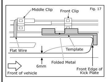
17. Fold the cardboard template provided in the kit and place it over the sheet metal edge of the door sill. The cut-out in the template should be aligned with the metal tab folded over the sheet metal just behind the front clip as shown. Position the Kick Plate so the forward edge touches the template as shown. The Kick Plate should be **6mm** from the outermost edge of the door sill.
