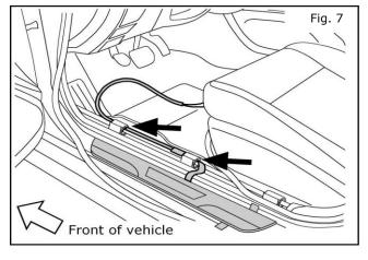
Place Illuminated Kick Plate into position on the driver side door sill. Feed the end of the wiring up through the existing harness clips towards the footwell.
