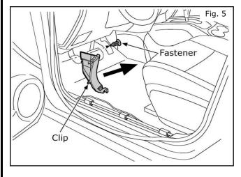
5. Remove one (1) fastener from the outer footwell trim panel (LH). Use a trim stick to carefully pry off the trim panel, pulling the part horizontally toward center of vehicle.
